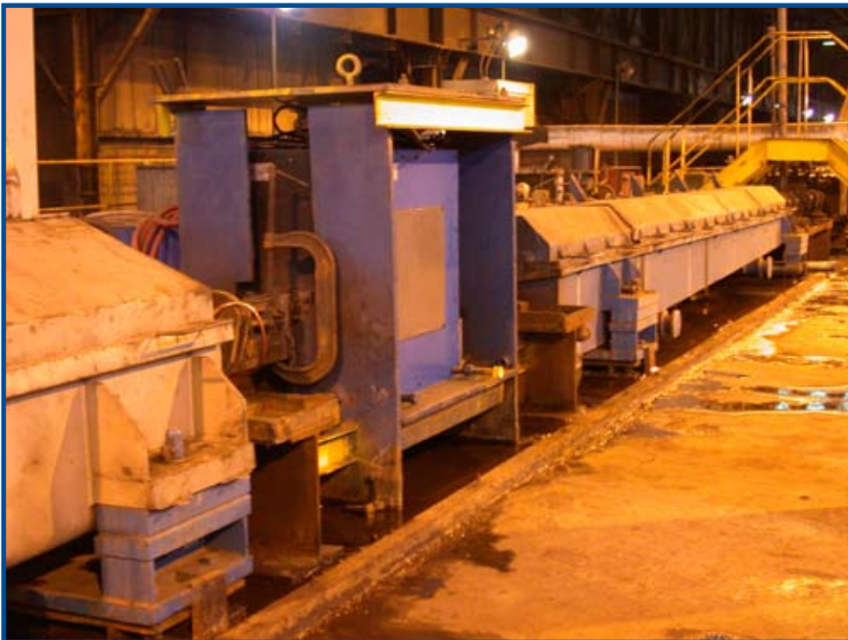
This first commercial prototype was used to test SQA™ program features. The system is installed in a steel rod mill, where rolling speeds exceed 60 meters per second.
